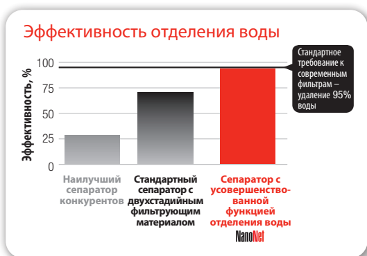
Modified SAE J1488 emulsified water removal test, mid-range diesel engine fuel/water separator, 15,000 miles in service.
